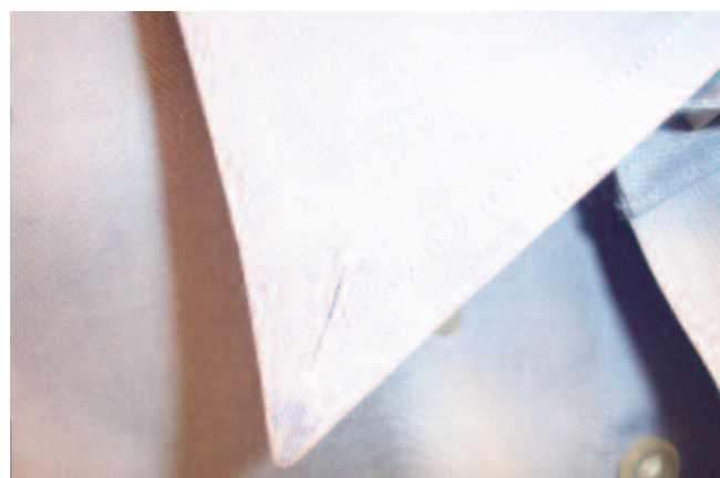
Substandard collar bonding agents can melt during normal professional cleaning, leaving glue stains similar to those on this collar.
