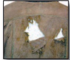
The selection of thin or weak skins during manufacturing can result in tearing during cleaning.
