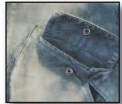
Exposure to light and natural elements can cause leather dyes to oxidize. Severe color losses are due to poor selection of dyes, oil, and finishes during the manufacturing process.
