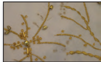
The decorative gold beads dissolved during proper drycleaning and stained the adjacent fabric areas.
